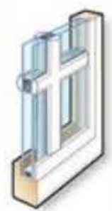
Permanent exterior and permanent interior with spacer
