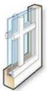
Permanent exterior and permanent interior without spacer
