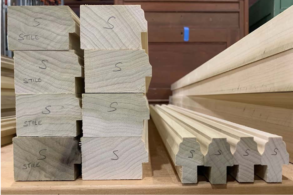
Poplar muntins, rails, and stiles of windows showing interior detail, and stain match.
