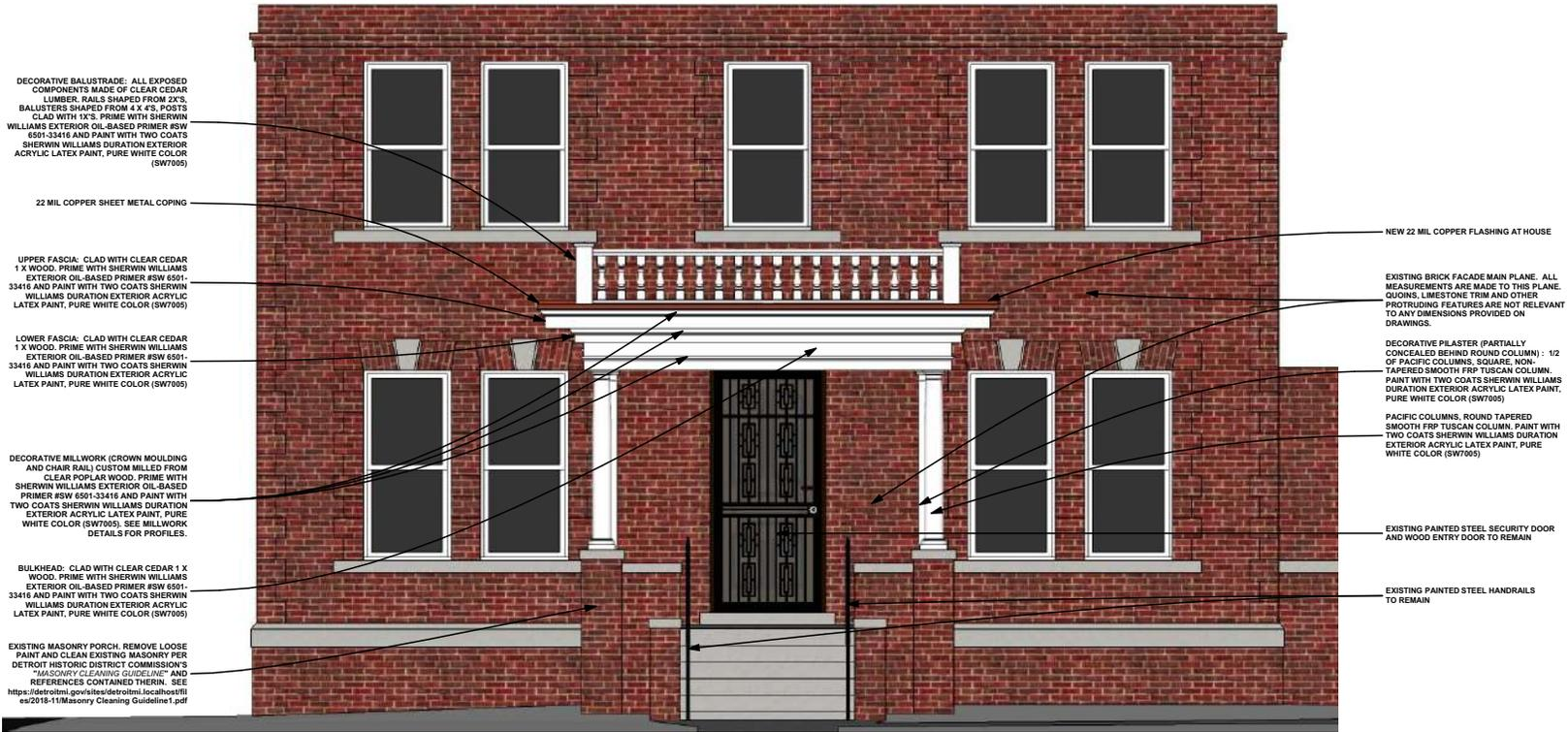
DECORATIVE BALUSTRADE: ALL EXPOSED COMPONENTS MADE OF CLEAR CEDAR LUMBER. RAILS SHAVED FROM 2X4S. BALUSTERS SHAPED FROM 4 X .4S. POSTS CLAD WITH 1X6S. PRIME WITH SHERWIN WILLIAMS EXTERIOR OIL-BASED PRIMER #SW 6501-33416 AND PAINT WITH TWO COATS SHERWIN WILLIAMS DURATION EXTERIOR ACRYLIC LATEX PAINT, PURE WHITE COLOR (SW7005)
