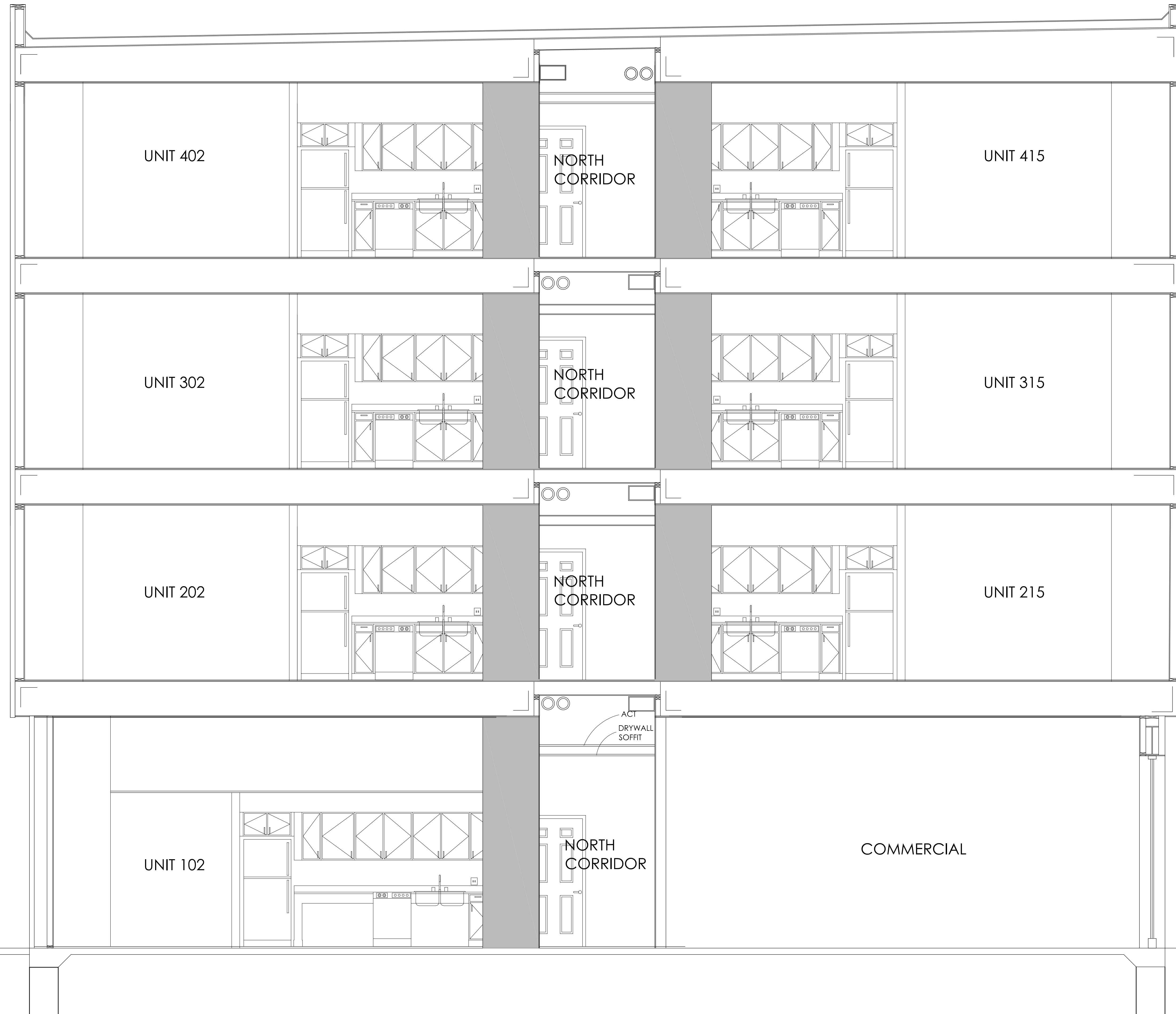
A BUILDING SECTION SCALE: 3/8"=1'-0"
