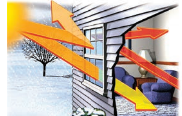
Winter Energy Savings: Low-E insulating glass reduces heat loss by reflecting warmth back into your home.
