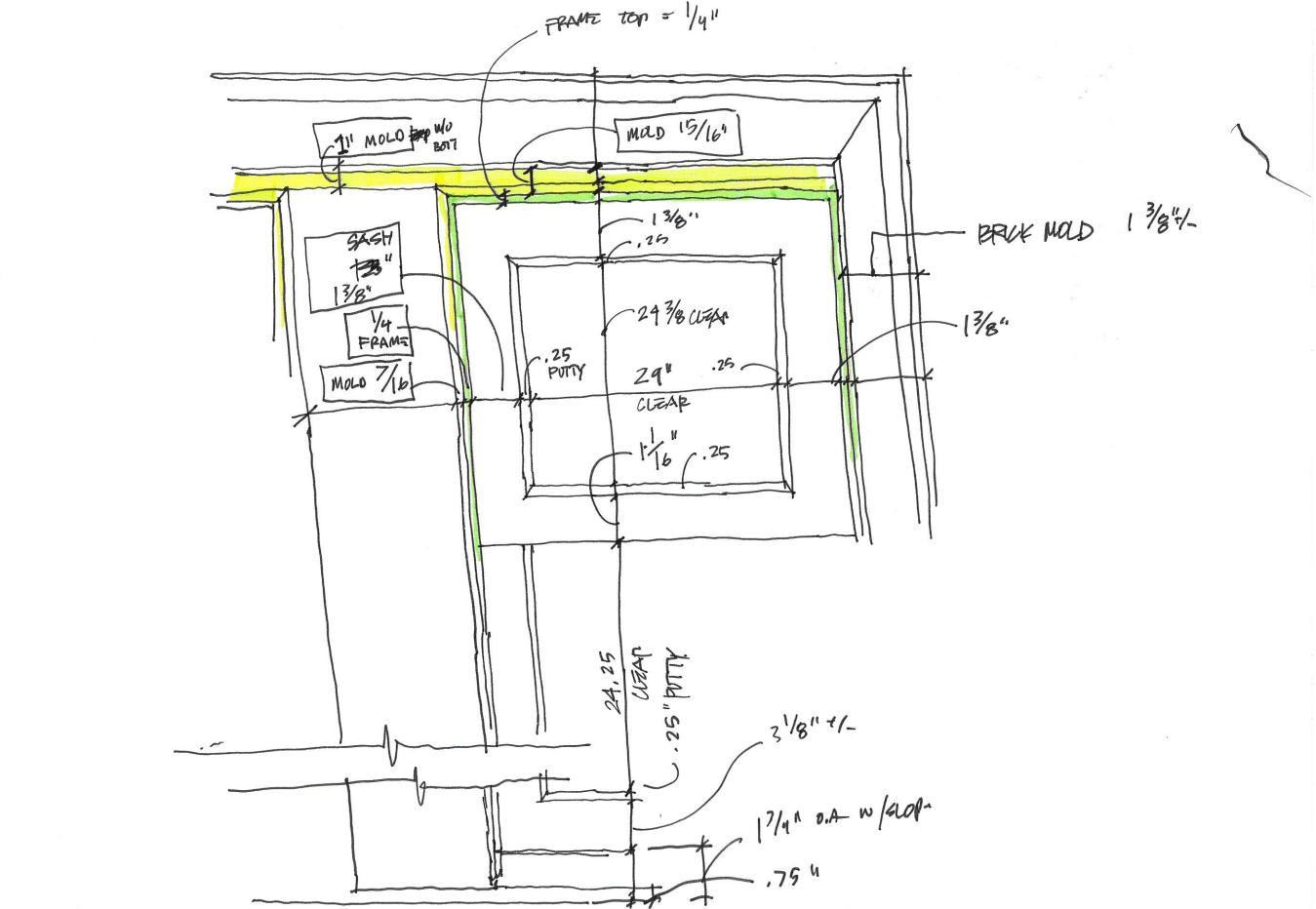
Detail of brickmould and location of window and sash in opening.
