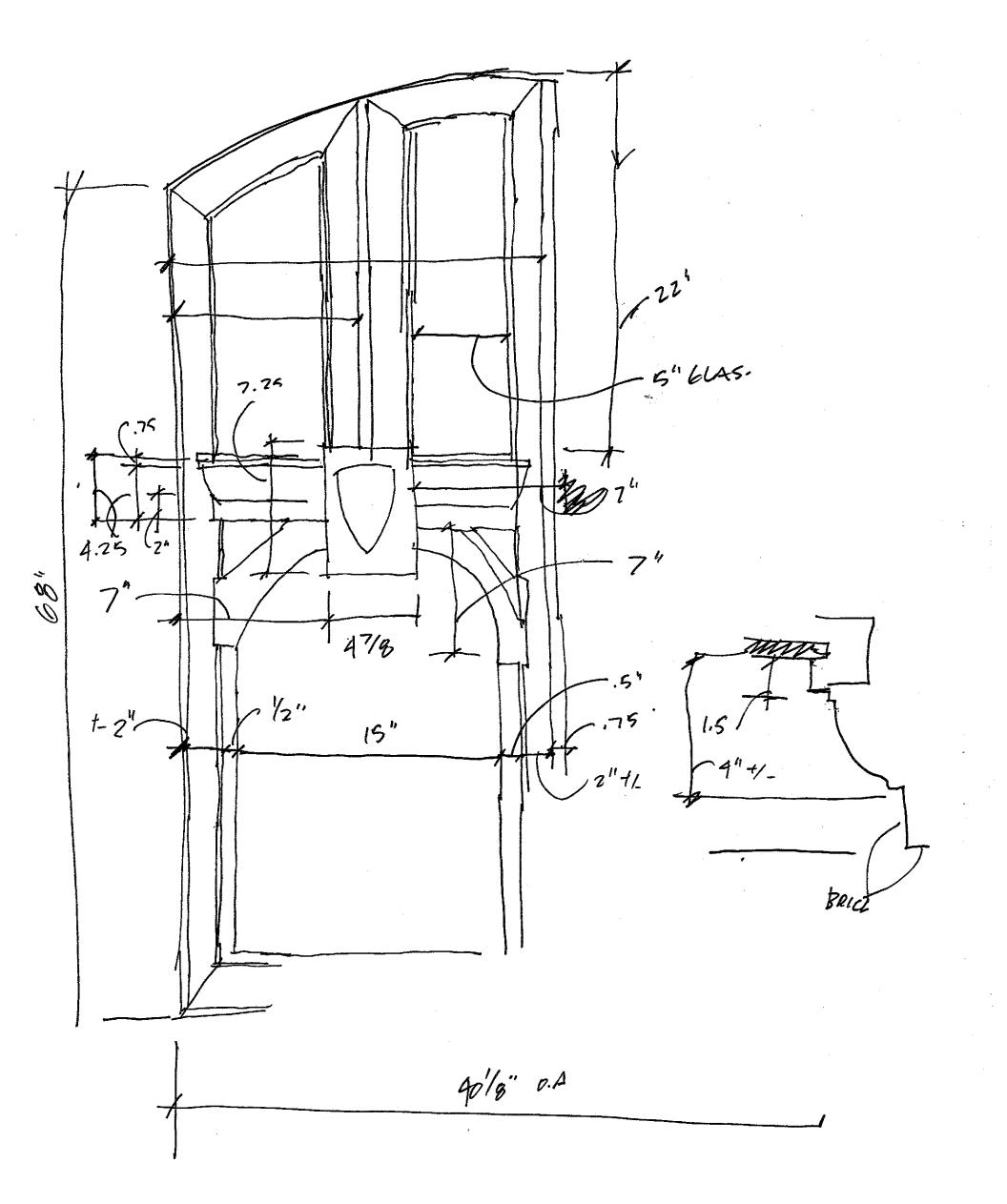
Detail of framing on all decorative windows. This specific section shows the glazing dimensions for the small window over the ramp, however the other windows have similar trim proportions. All trim will be replicated as existing with missing portions being added to the systems.
