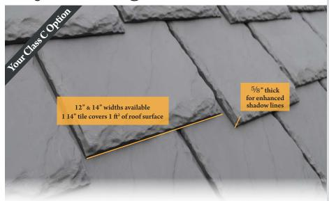
**B**igger is better when it comes to EcoStar LLC's latest innovation. Majestic Niagara Slate is a natural-looking, 5/8" thick, synthetic slate roofing tile produced in 12" and/or 14" widths. This added size allows each Majestic Niagara Slate 14" tile to cover one square foot of roof deck at the 10" exposure (100 tile/square), maintaining a 2" headlap throughout. An additional 9" exposure option allows for the creation of unique looks using staggered, offset or random width installations.
