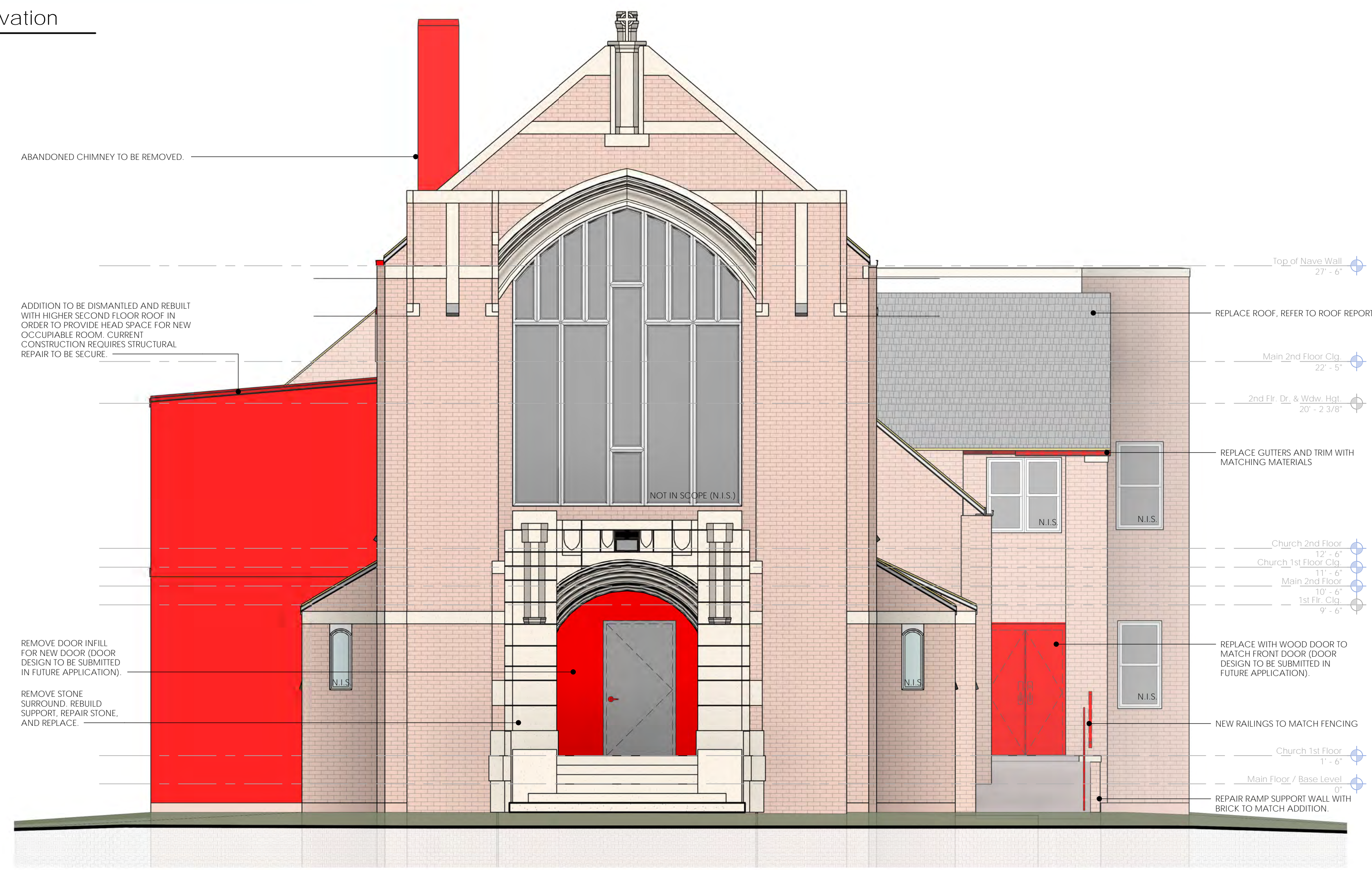
1 Demo Front (North) Elevation 1/4" = 1'-0"
