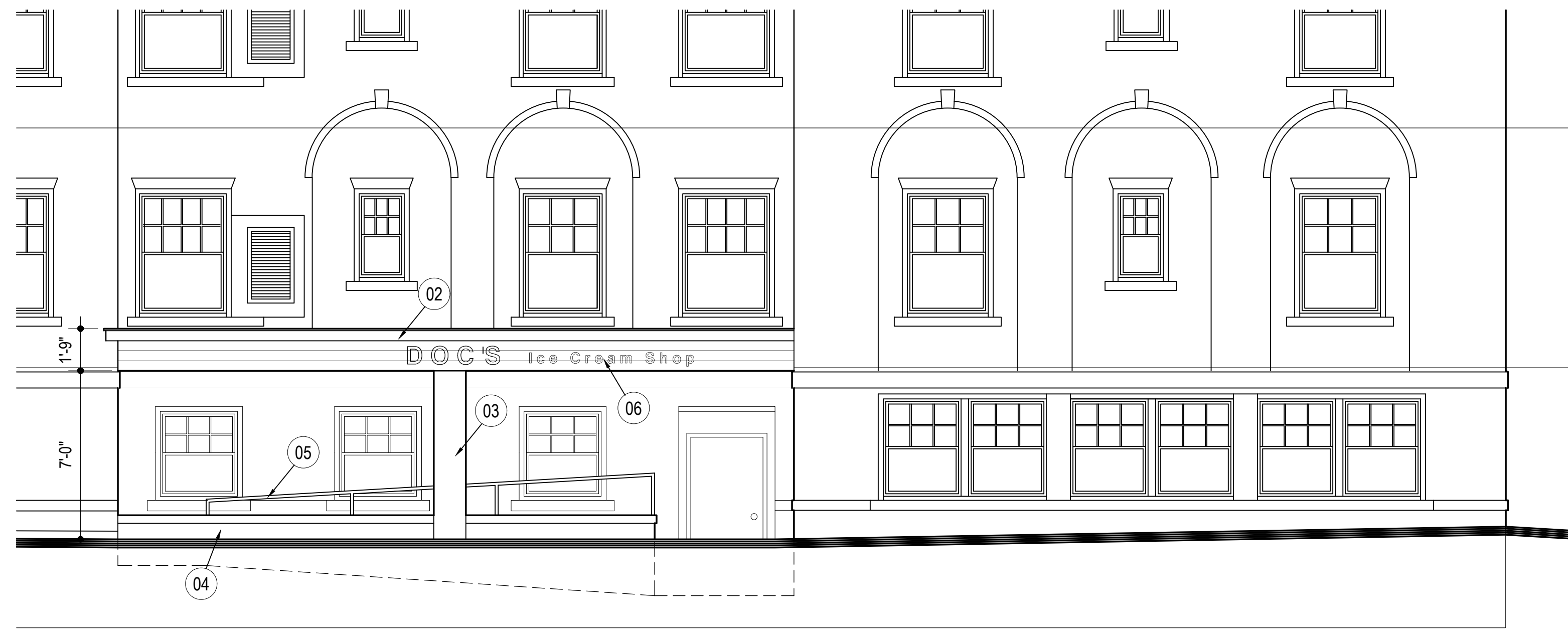
3 PARTIAL EAST ELEVATION AT NEW CANOPY A-1 1/4"=1'-0"
