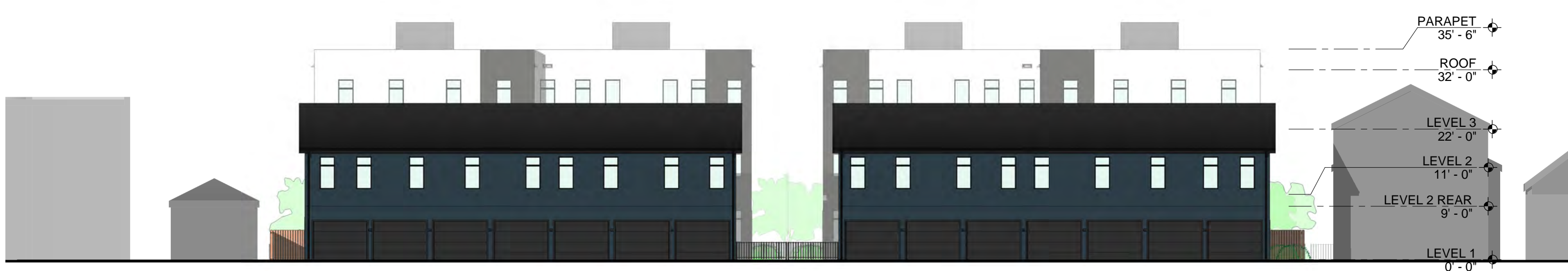
N GARAGE NORTH ELEVATION (YARD) 1/16" = 1'-0"
