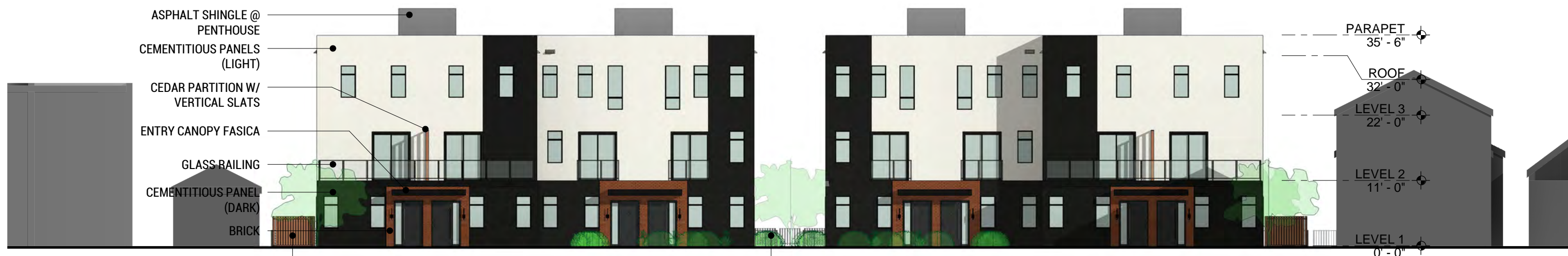
N BAGLEY NORTH ELEVATION (YARD) 1/16" = 1'-0"
