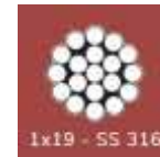
Stainless Steel Wire Rope 1/8" Dia. Breaking Strength = 1,780 Lbs Weight Per 100' = 3.3 Lbs 1/4" Dia. Breaking Strength = 6,900 Lbs Weight Per 100' = 13.5 lbs
