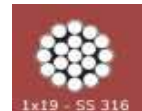
1x19 - SS 316 Stainless Steel Wire Rope 1/8" Dia. Breaking Strength = 1,780 Lbs Weight Per 100' = 3.3 Lbs 1/4" Dia. Breaking Strength = 6,900 Lbs. Weight Per 100' = 12.5 lbs
