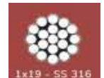
1x19 - SS 316 Stainless Steel Wire Rope 1/8" Dia. Breaking Strength = 1,780 Lbs Weight Per 100' = 3.3 Lbs 1/4" Dia. Breaking Strength = 6,900 Lbs. Weight Per 100' = 12.5 lbs
