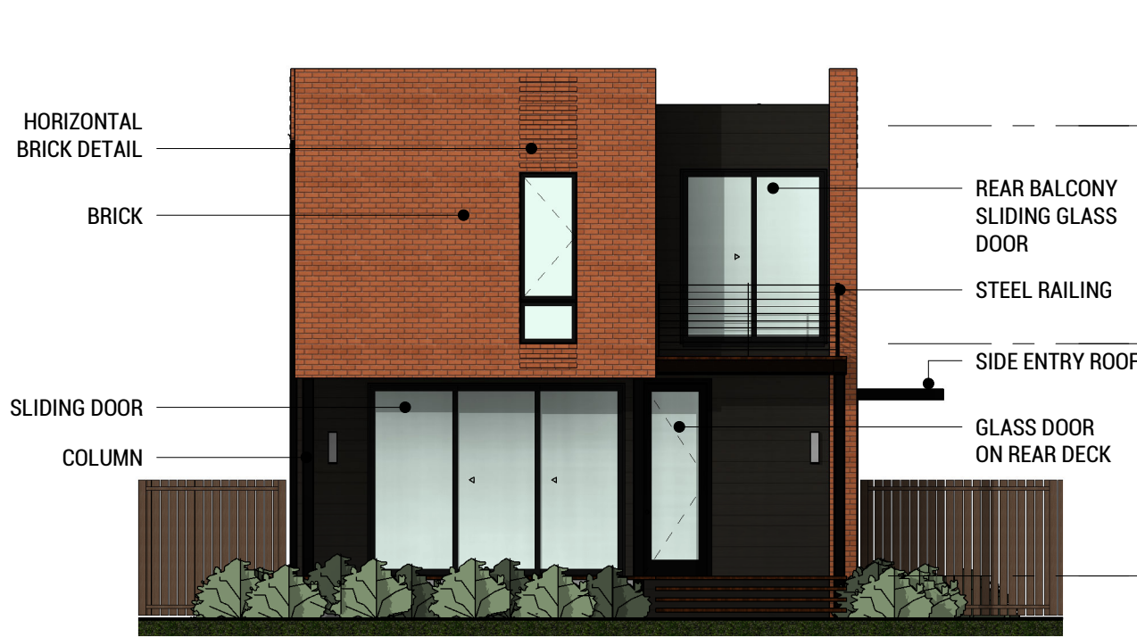
W WEST ELEVATION (REAR) 1/8" = 1'-0"
