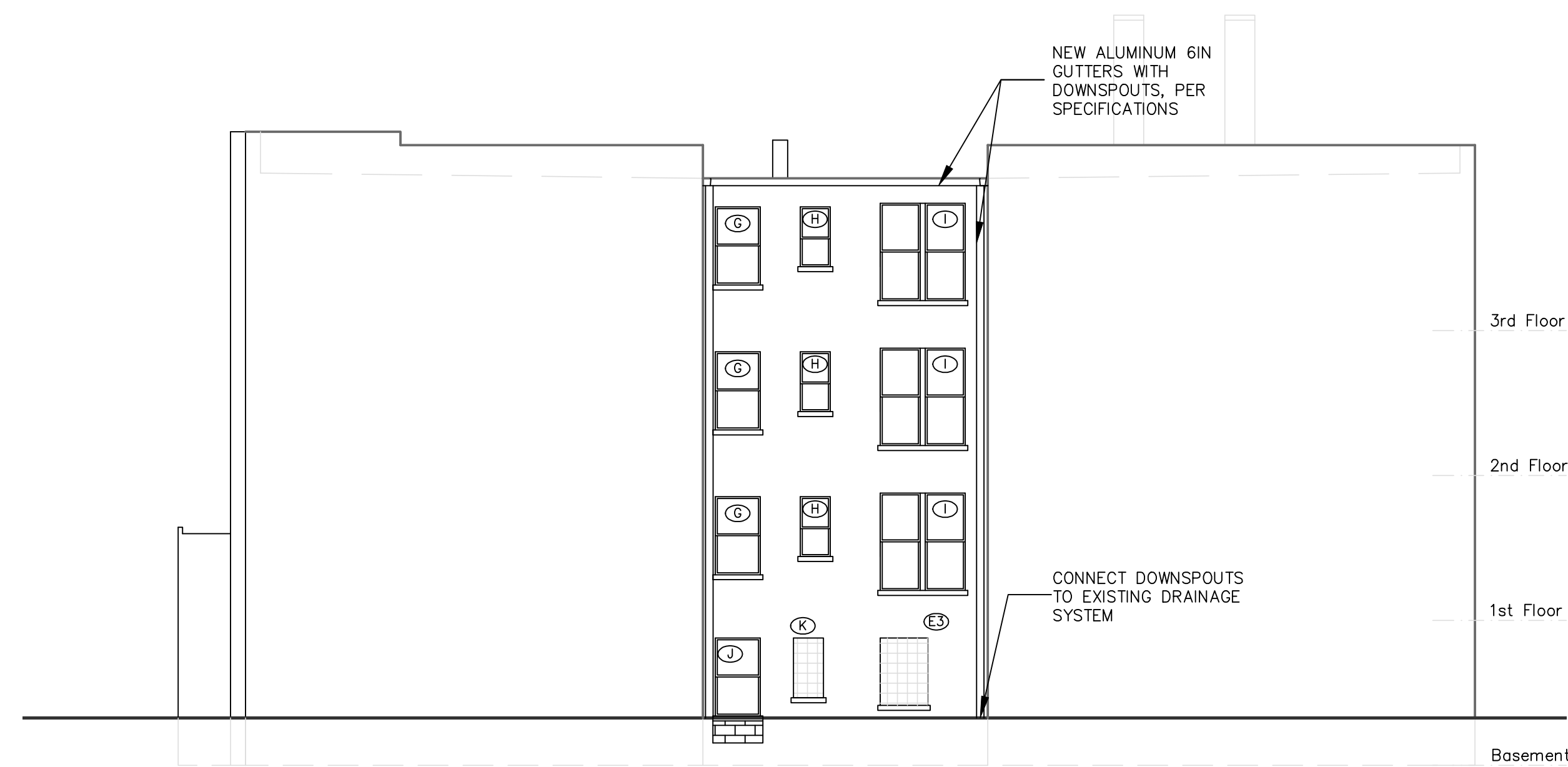
N BUILDING ELEVATION – NORTH A1/A6 1/4" = 1'-0"
