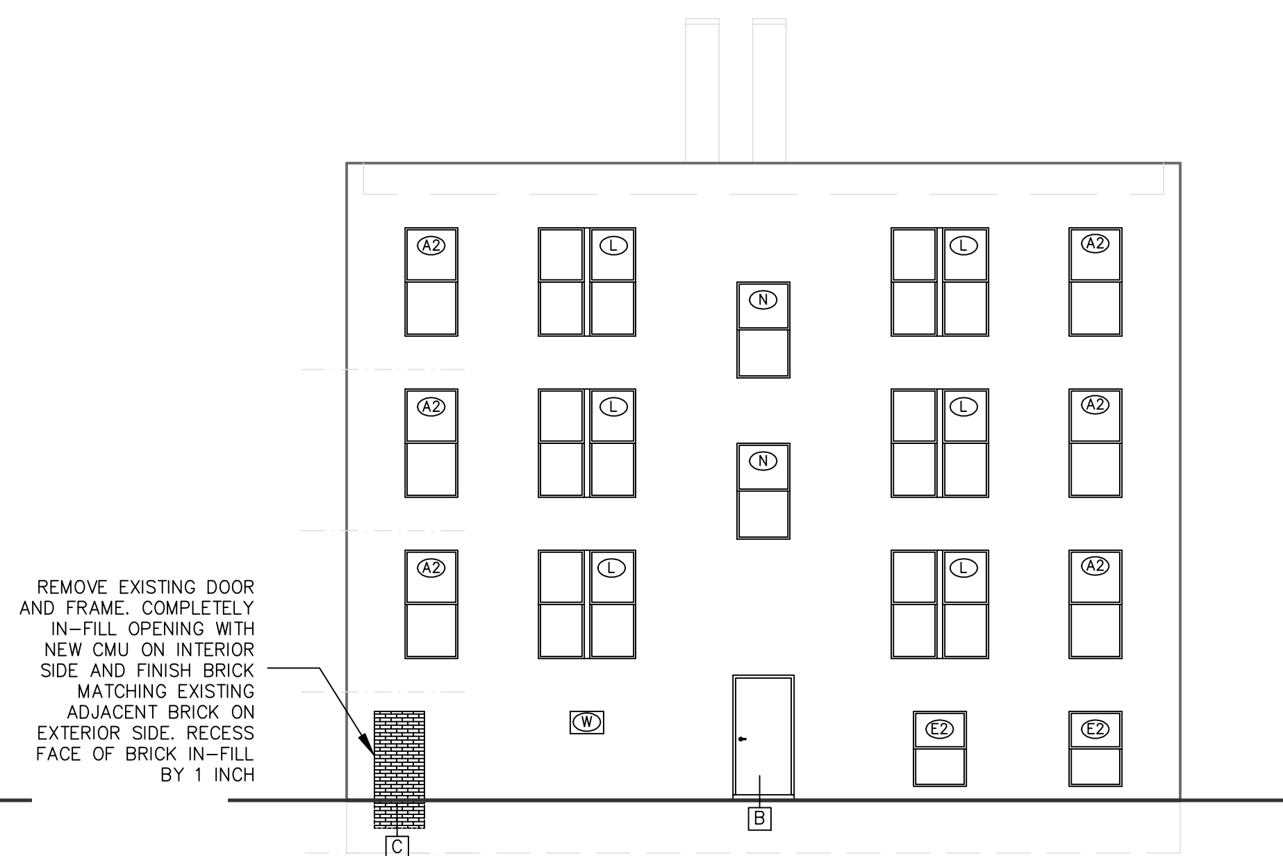
W BUILDING ELEVATION – WEST A1/A6 1/8" = 1'-0"
