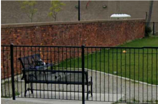
6' ht. Screen Wall - Brick to match Architecture
