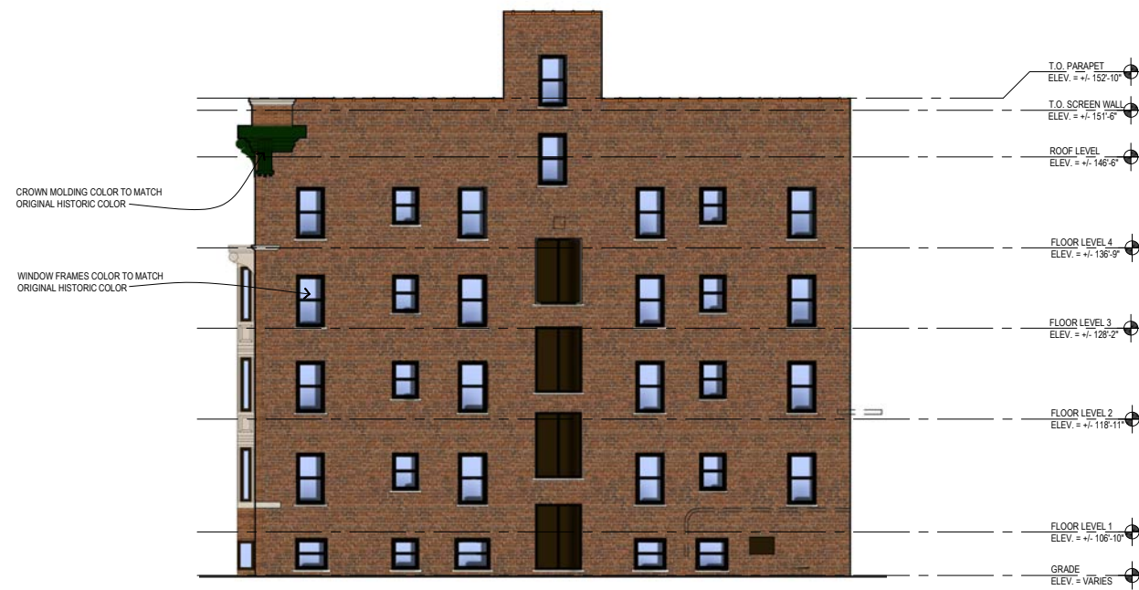
WEST EXTERIOR ELEVATION
