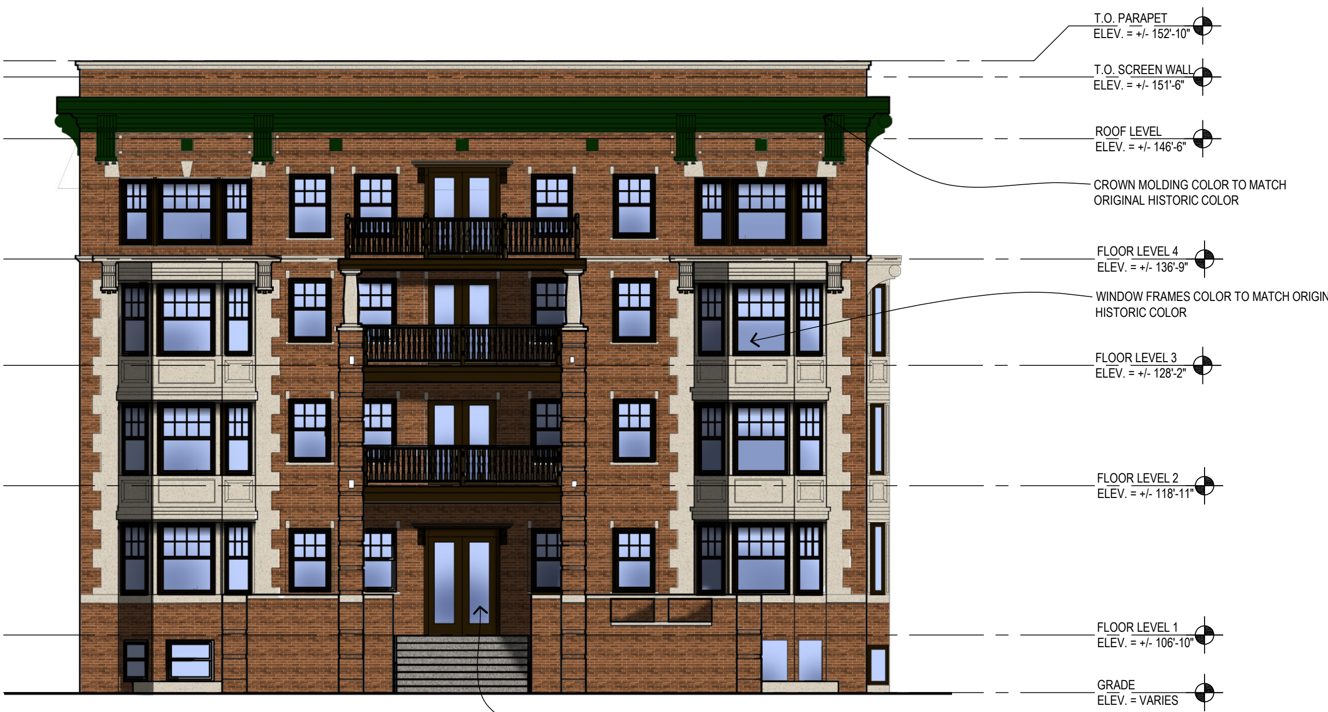
1 6A401.1 2467 CASS EAST EXTERIOR ELEVATION 1/8" = 1'-0"
