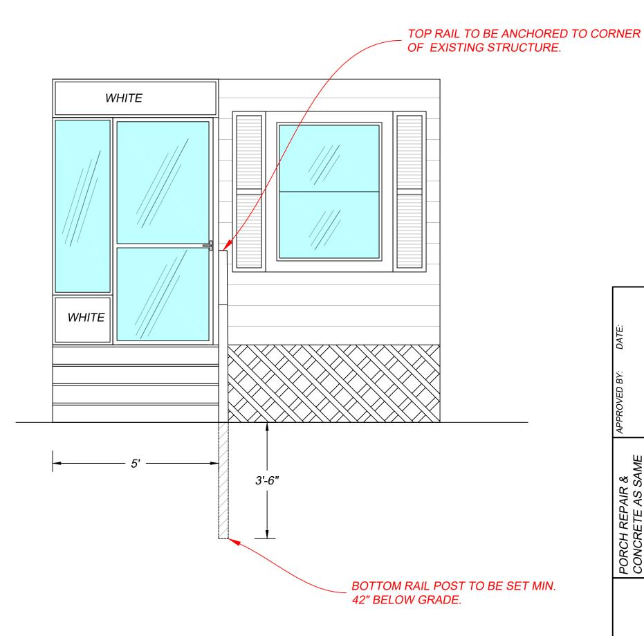
MRC R311.7.7 REQUIRES AT LEAST ONE HANDRAIL PROVIDED ON ONE SIDE OF CONTINUOUS RUN OF TREADS OR FLIGHT WITH FOUR OR MORE RISERS.
