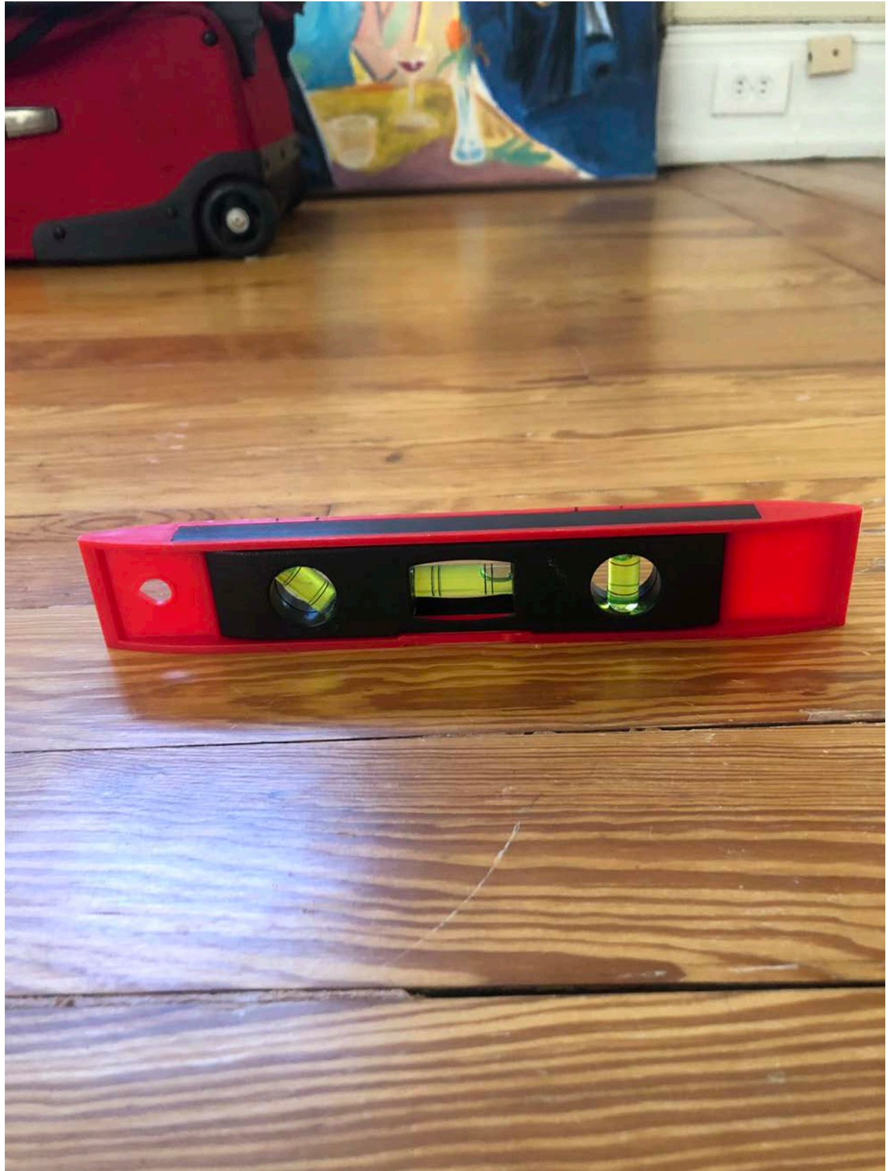
2ND FLOOR PITCH DUE TO SETTLING
