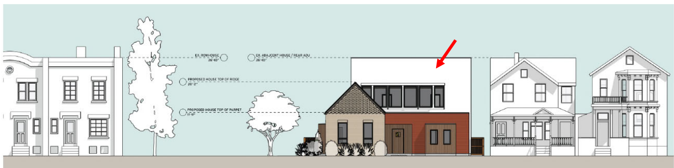
Bagley Street elevation, with roof heights labeled. Proposed new construction is in color, existing in white. Applicant images.
