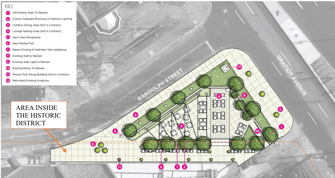
Figure 3 by Applicant: Gratiot Plaza Plan, showing the proposal. Changes include closing off opening to Randolph and Gratiot corner with new wall, moving sculpture to the corner from the center of the plaza, adding a new stair to the middle center of the plaza, and adding festoon/ overhead lighting, tables, and chairs. The area below the dashed orange line includes the portion of the plaza/outlines the work which is located with the district's boundaries. The area of the plaza above the dashed orange line is outside of the district. Therefore, only the proposed work below the dashed orange line is subject to HDC review while the area of work above the dashed
