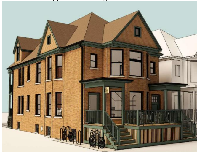
Staff confirmed with the applicant that the side bay windows are drawn incorrectly on the rendering (transom and fixed window in central openings will remain)
