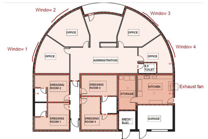
Figure 2, by applicant, floor plan showing locations of the window replacement and vent installation.
