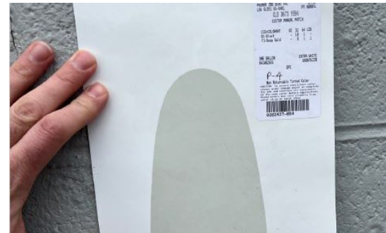
Site Photo 3, by applicant proposed paint against existing wall, showing slight lighter gray shade than existing.
