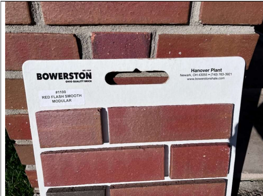
Photo 9 Manufacturer board for brick, same brick used to build garage
