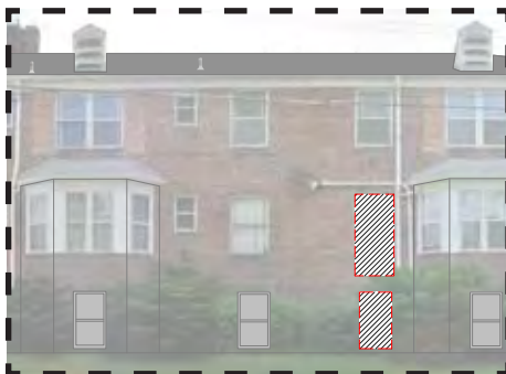
Demolition Elevation @ New Accessible Entry
