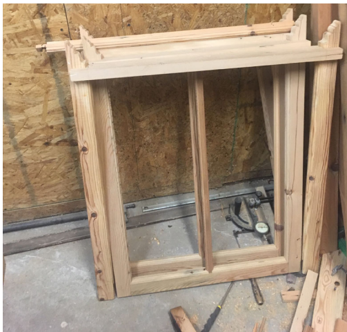
Custom-built wood windows proposed for the house.
