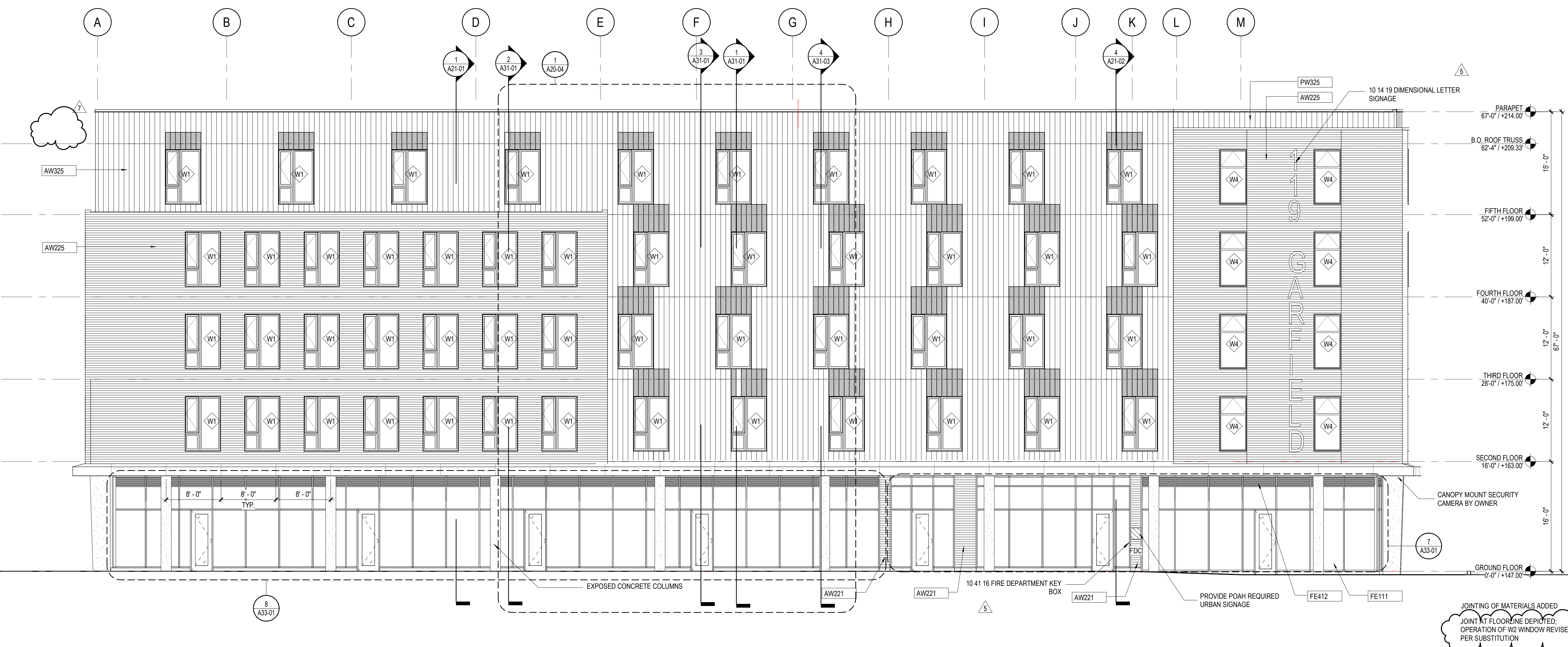
1 SOUTH ELEVATION- GARFIELD STREET 1/8" = 1'-0"
