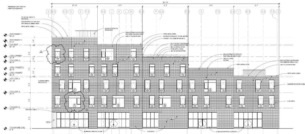
The proposed revised elevation, per submitted drawing A3.1.1. The proposed type brick “BR-1” is the same on all sides of the building. Notice the markedly inconsistent parapet heights (the dimension between the tops of the highest windows, and the tops of each mass).
