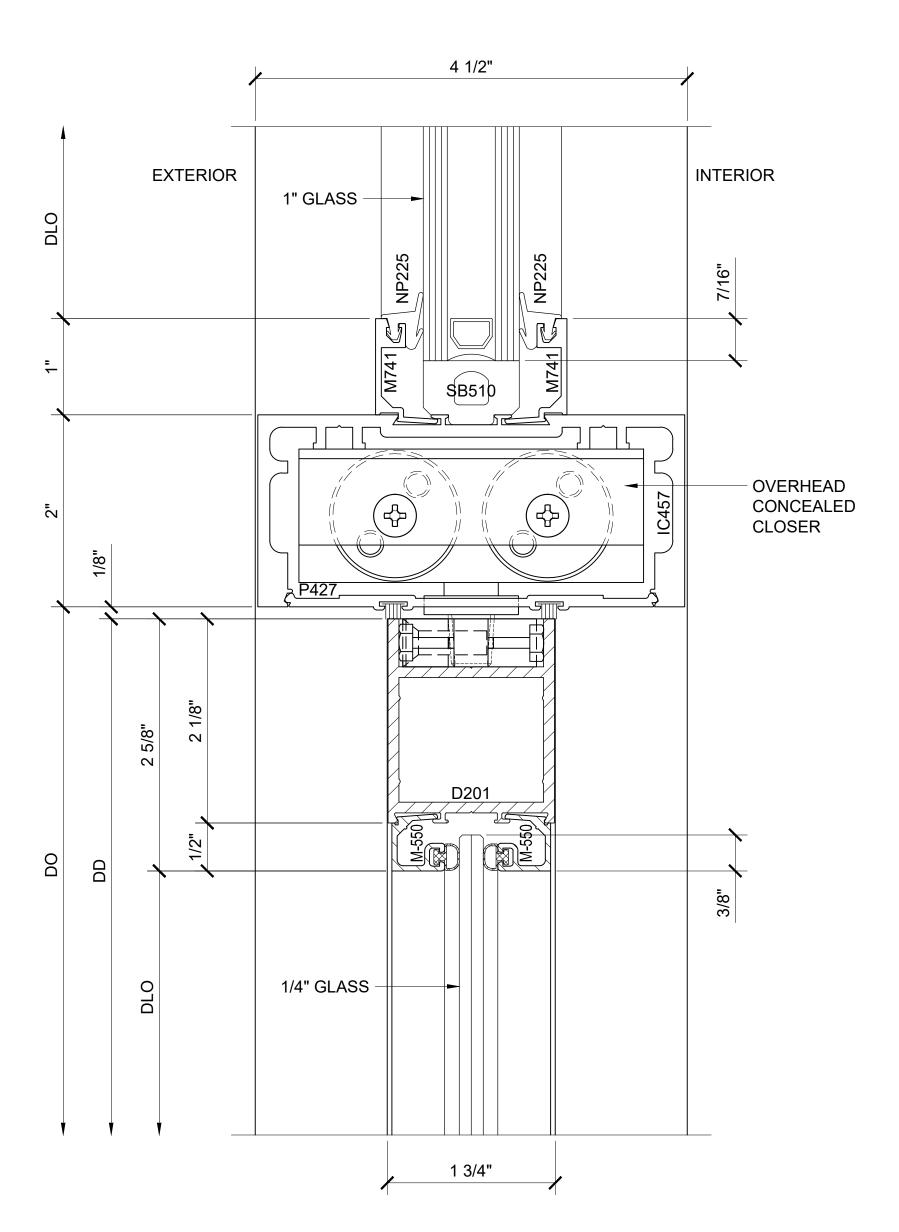
SECTION DETAIL @ DOOR HEAD WITH PIVOT (2)
