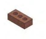
**2 1/4 Modular** – This brick size is the industry standard. It was designed to fit to a mason's hand grip. The unit is designed to turn corners and start a wall in running bond (this is where the mortar joints in the brick below are centered on the brick above). 3 brick courses equals one brick laid in a soldier course (stacked vertically). This brick is the easiest to use when creating patterns in the wall There are 6.85 brick per square foot.
