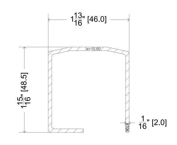
STEEL REINFORCEMENT 8706 @ SASH
