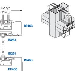
Exterior face of 1/4" (6) glazing aligns with exterior face of 1" (25) glazing
