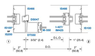
\*NOTE: IS100 Insert is required to install glass between doors
