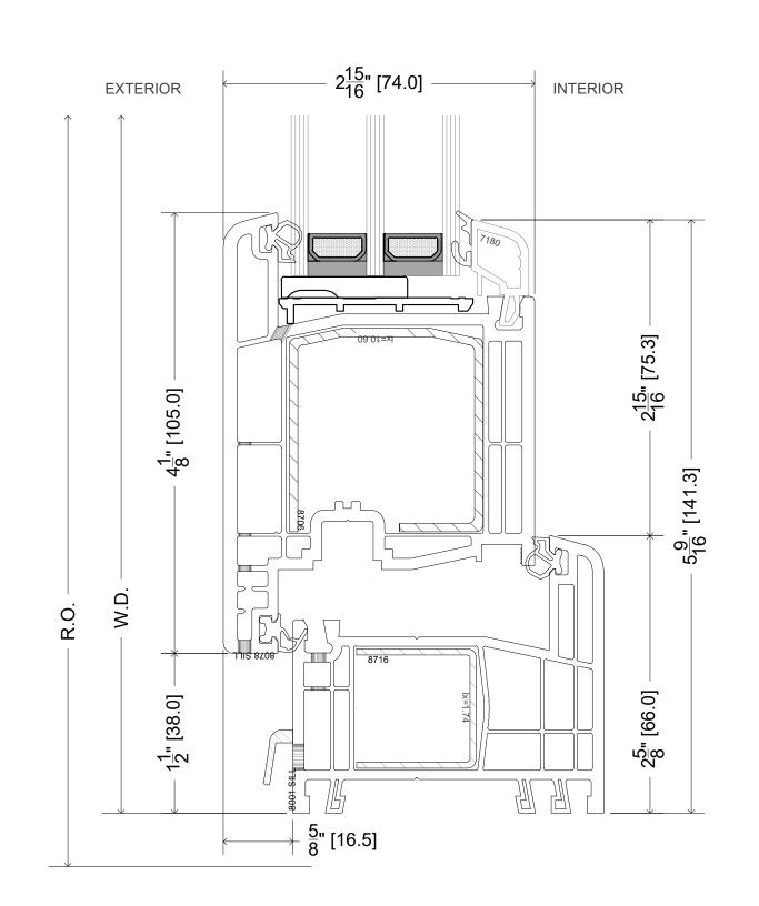
3 AWNING WINDOW SECTION PROFILE @ SILL SCALE 1'-0" = 1'-0"
