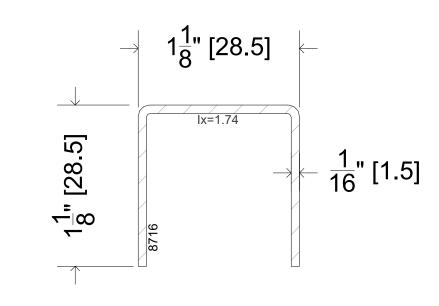
STD. STEEL REINFORCEMENT 8716 @ SASH SCALE 1'-6" = 1'-0"
