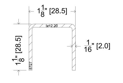
STEEL REINFORCEMENT 8727 @ SASH SCALE 1'-6" = 1'-0"
