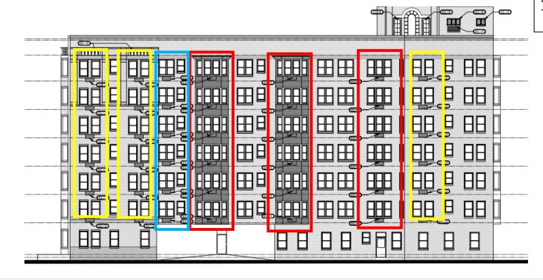
Notes indicates **EXISTING VENTS** and **NEW VENTS** at this elevation which were **APPROVED BY THE COMMISSION IN 2019. NEW VENTS** are proposed at these three columns (outlined in yellow) WITH THE CURRENT 2021 PROPOSAL.
