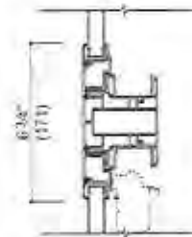
Vertical Section Transom over Single-Hung
