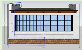
Area outlined in blue indicates the portions of the walls that will be replaced in kind (entire south wall and parapet and bottom portion of the west wall)
