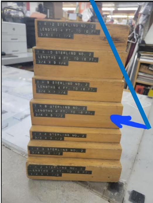
All fascia board will be made from 1 x 6 Tongue in Groove wood board for the front, rear and sides of the home.
