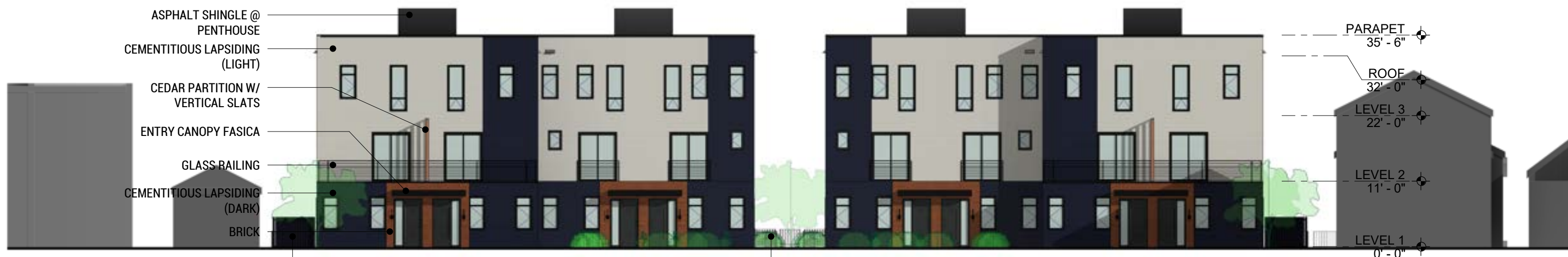
N BAGLEY NORTH ELEVATION (YARD) 1/16" = 1'-0"
