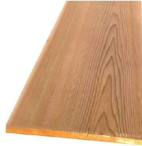
1 X WESTERN RED CEDAR BOARDS #2 AND BETTER USED TO CLAD ALL FASCIAS AND EXPOSED FRAMING AND PAINTED.
