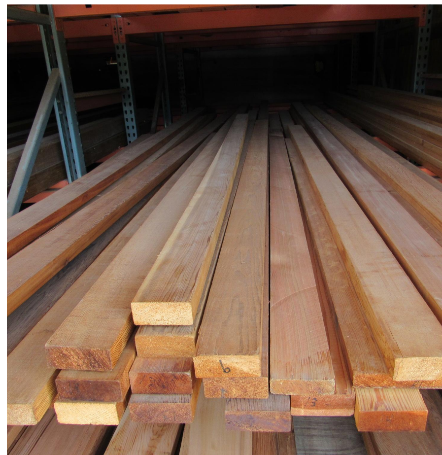
2 X WESTERN RED CEDAR LUMBER #2 AND BETTER TO BE SHAPED FOR HORIZONTAL MEMBERS OF BALUSTRADE AND PAINTED
