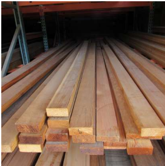
2 X WESTERN RED CEDAR LUMBER TO BE SHAPED FOR HORIZONTAL BALUSTRADE MEMBERS AND POST CAPS (TO BE PAINTED)
