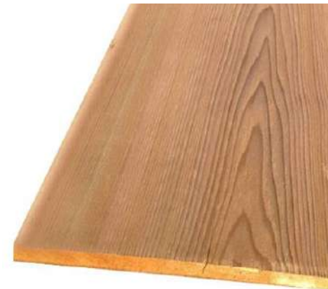
1 X WESTERN RED CEDAR BOARDS USED TO CLAD BALUSTRADE POSTS (TO BE PAINTED)
