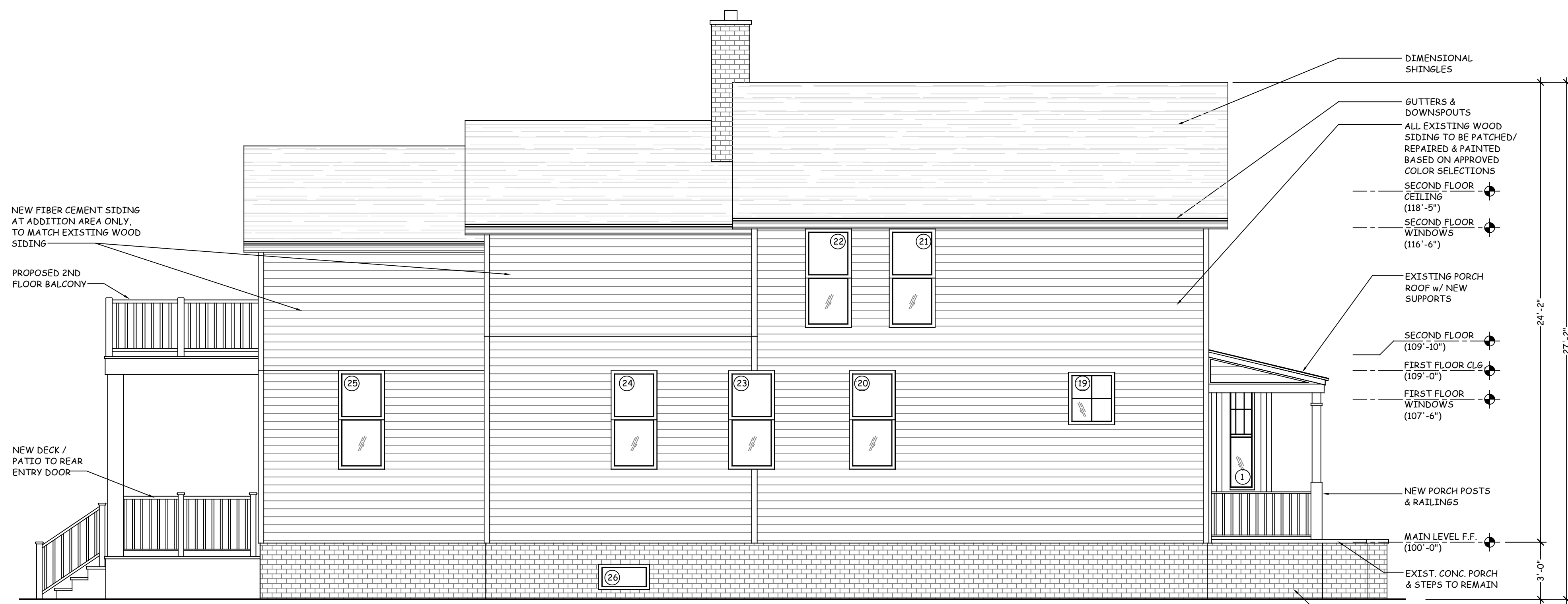
PROPOSED LEFT SIDE ELEVATION 'M' SCALE: 1/4" = 1'-0"
