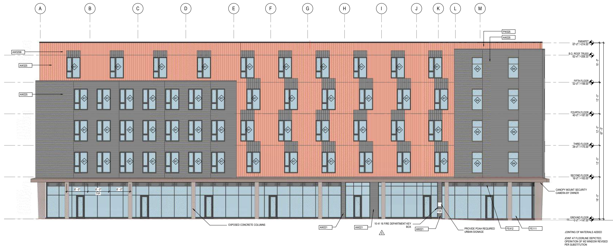
① SOUTH ELEVATION- GARFIELD STREET 1/8" = 1'-0"
