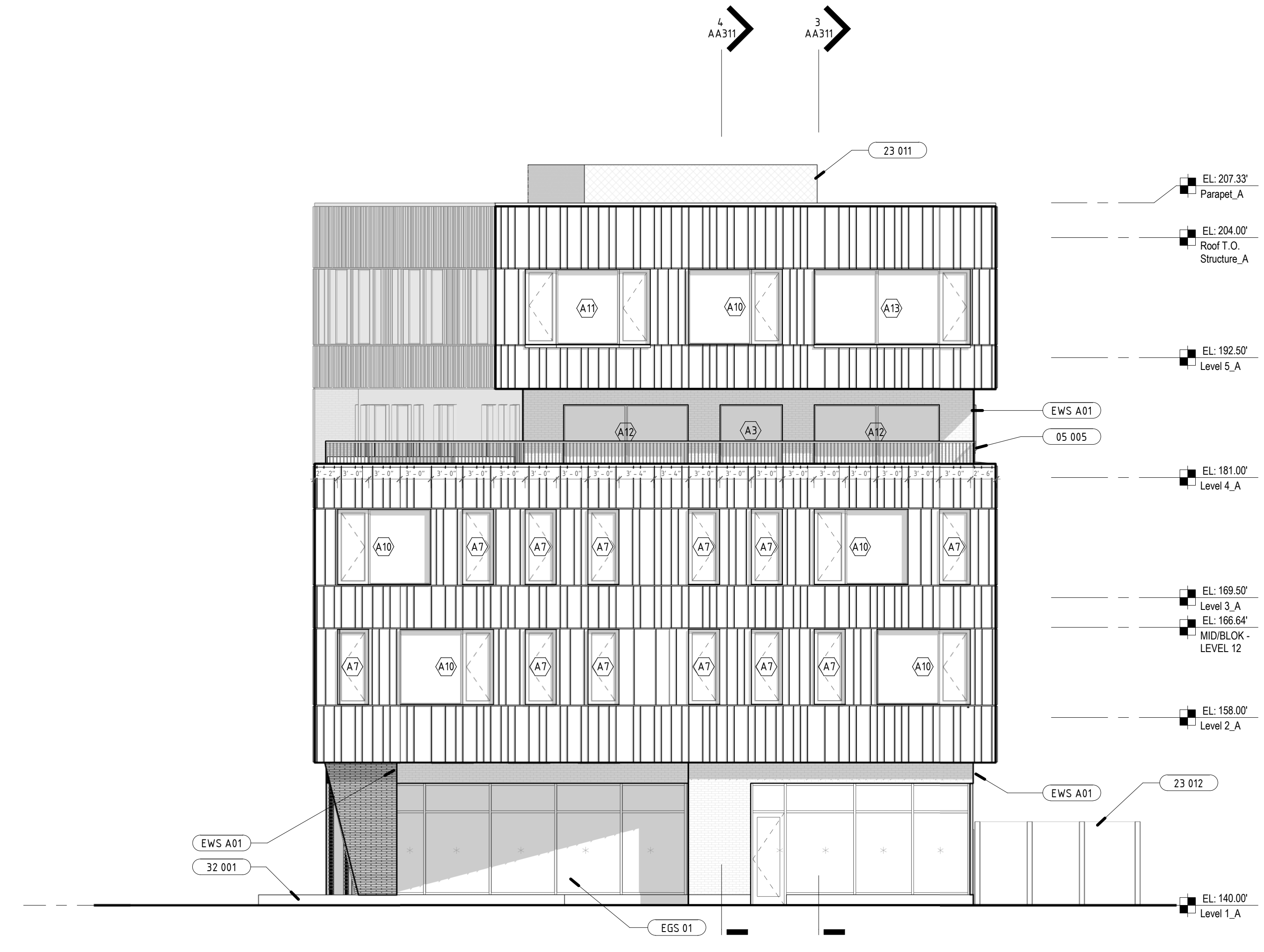
3 BUILDING A - SOUTH ELEVATION Scale: 1/8" = 1'-0"
