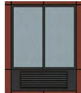
hvac ventilation louver at window FLUSH (NON-PROJECTING) ALUMINUM - BLACK
