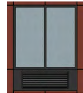
hvac ventilation louver at window FLUSH (NON-PROJECTING) ALUMINUM - BLACK
