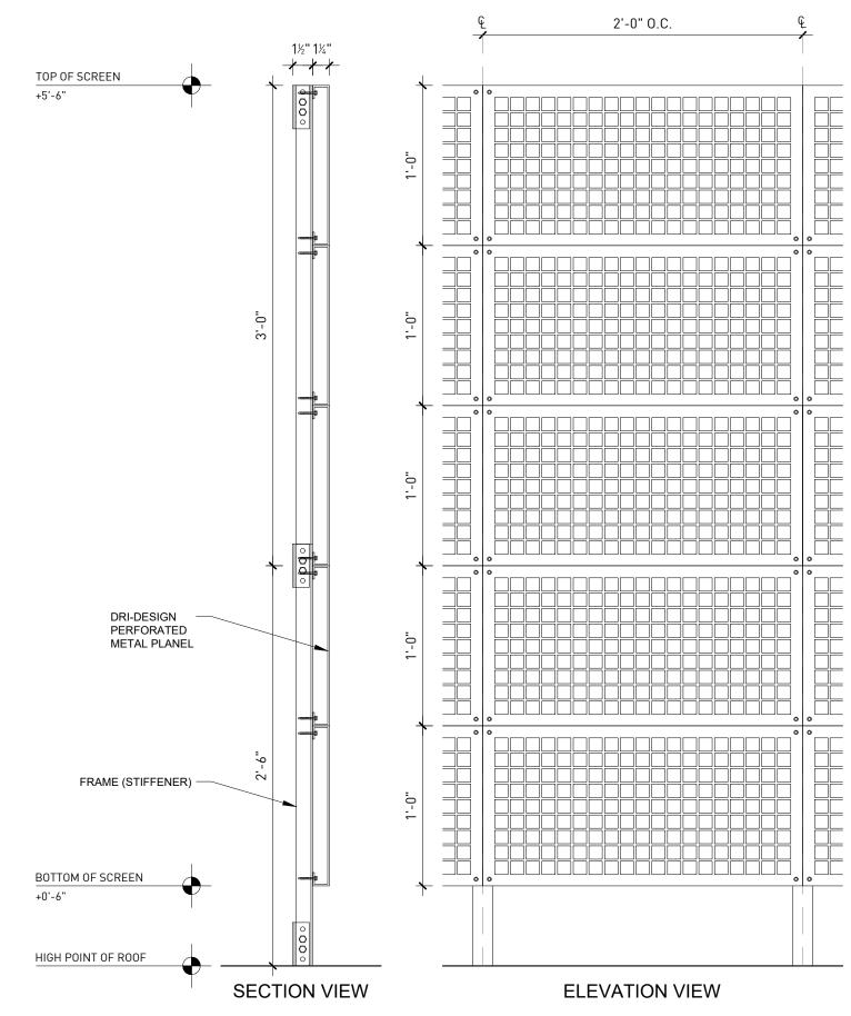
MECHANICAL EQUIPMENT SCREEN DETAILS "DRI-DESIGN, PERFORATED PANEL SERIES" ORIGINAL IMAGE SCALE: 3" = 1'-0"
