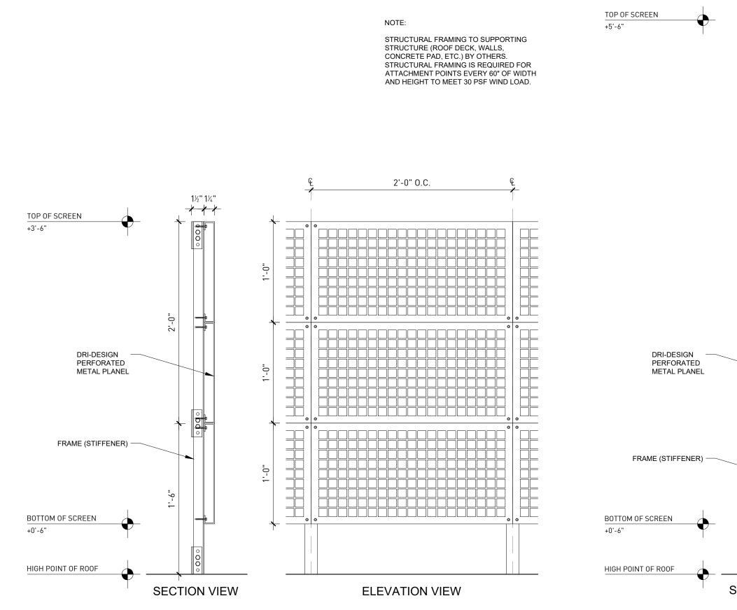
MECHANICAL EQUIPMENT SCREEN DETAILS "DRI-DESIGN, PERFORATED PANEL SERIES"
