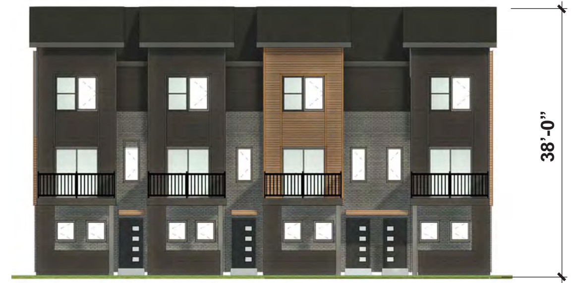
FRONT ELEVATION (16' WIDE UNIT - 4 UNIT BUILDING)
