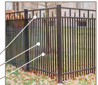
1.25" X 1.375" REINFORCED RAIL 0.75" PICKETS 1.5" SPACING (OPTIONAL)
