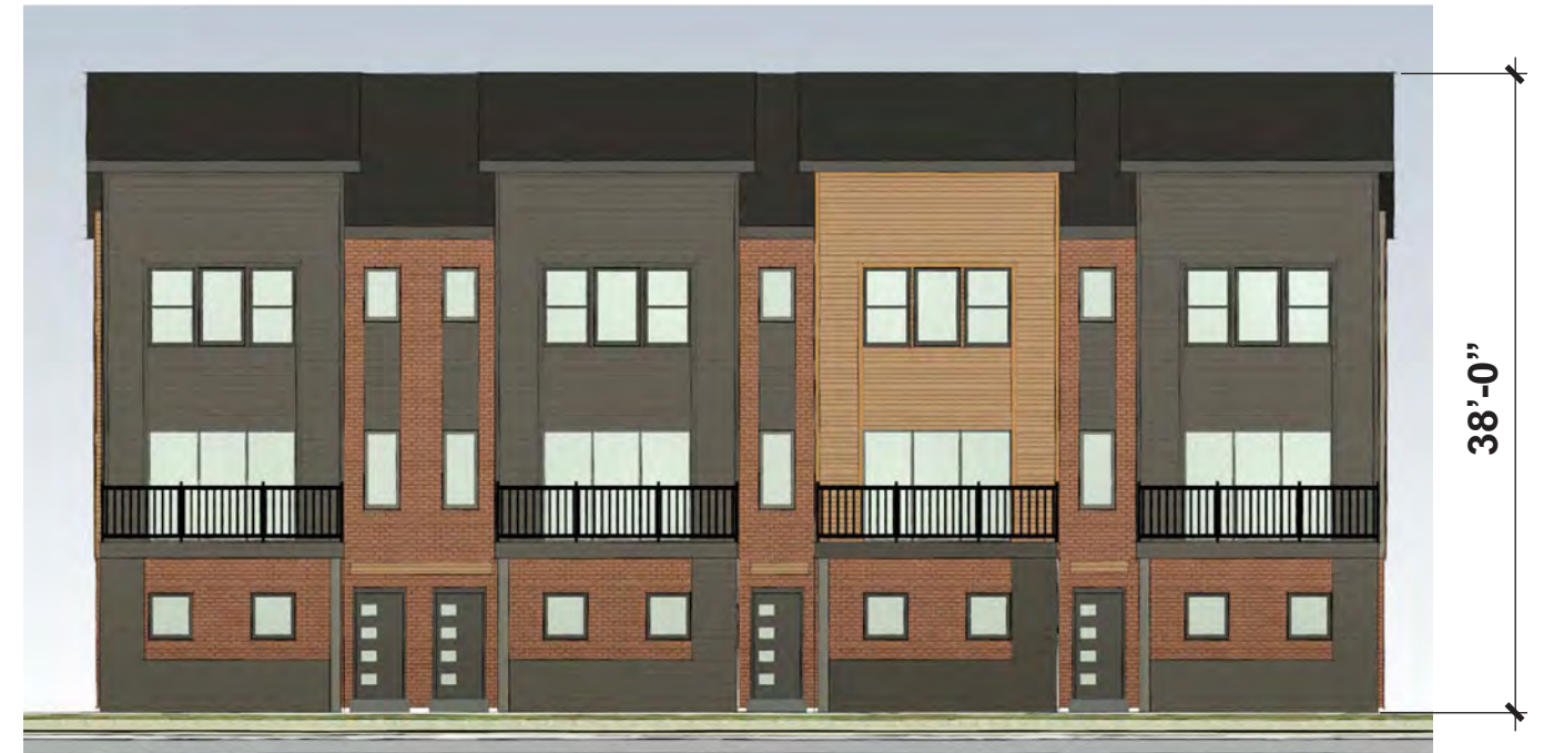
FRONT ELEVATION (20' WIDE UNIT - 4 UNIT BUILDING)
