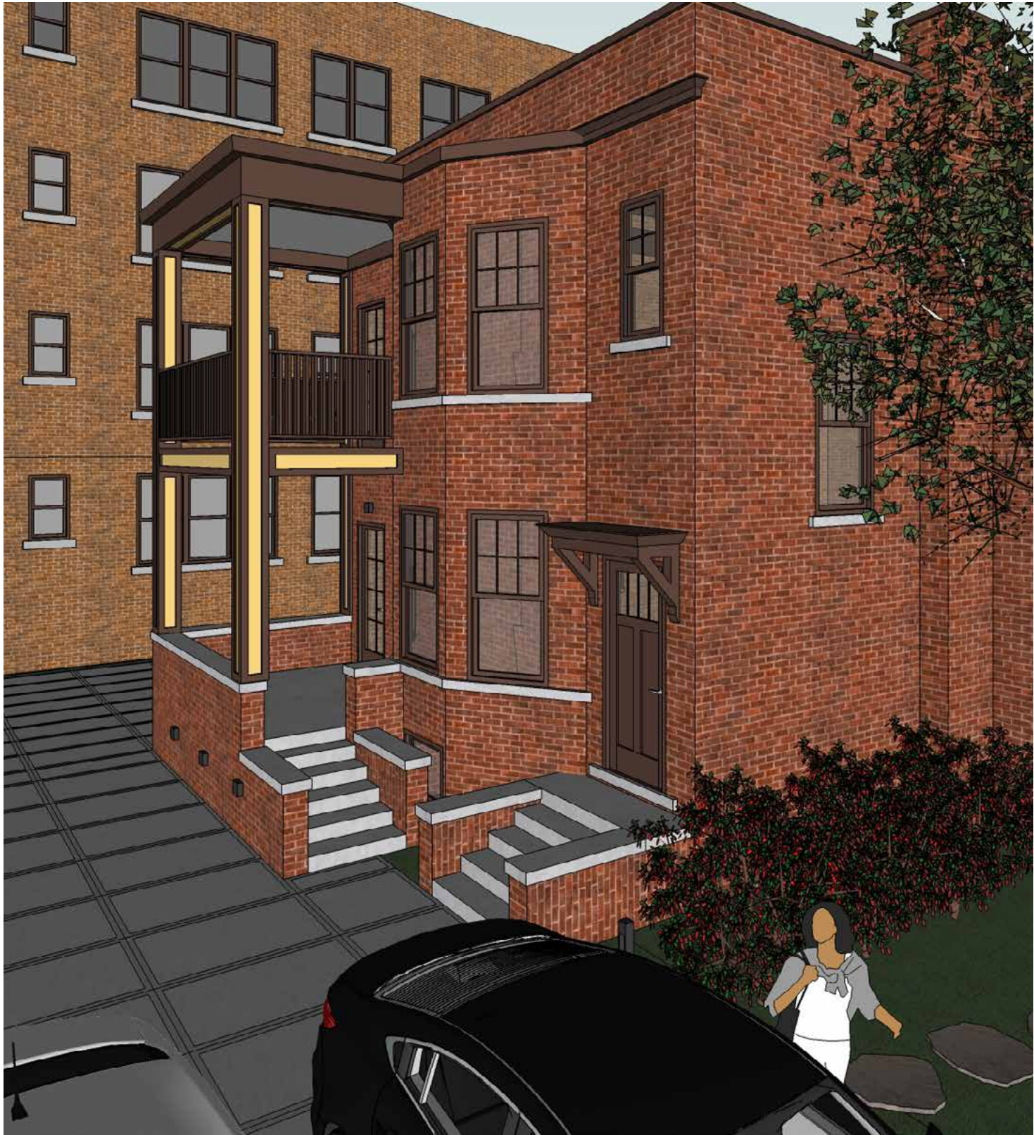
PROPOSED REINSTALLATION OF THE ENTRANCE STEPS TO PROVIDE CLEARANCE FOR THE DRIVEWAY
