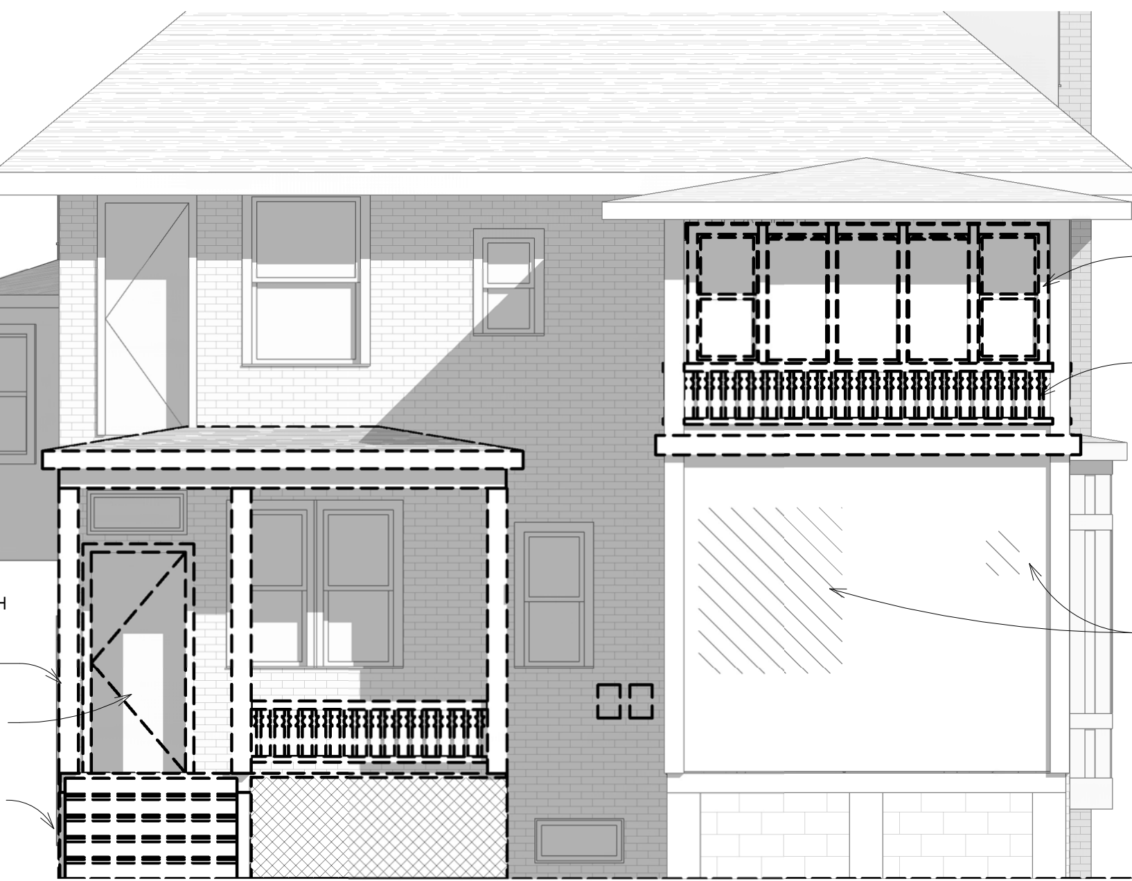
6 WEST ELEVATION - DEMO 1/4" = 1'-0"
