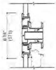
Vertical Section Transom over Single-Hung
