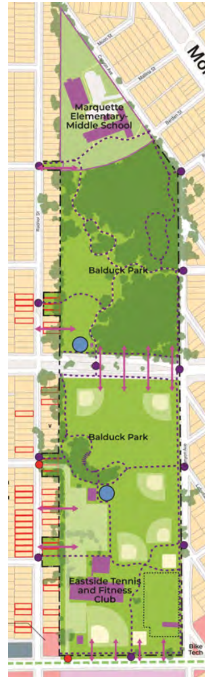
Figure 15: Initial concept plan for Balduck Park focusing on increasing access to an within the park, identifying gathering spaces, and, upgrading existing assets.
