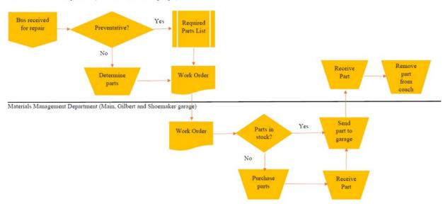
The flowchart ends with the mechanic removing the part from the coach because the disposition of the parts is unknown.
