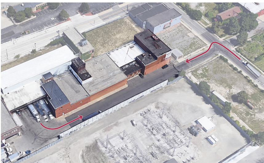
Rivard St (right) is wide enough for semi-trailers, while Brewster St (left) is too tight and leads trucks to encroach on the sidewalk. Photos: Google Earth
