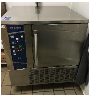
Exterior of Blast Chiller
