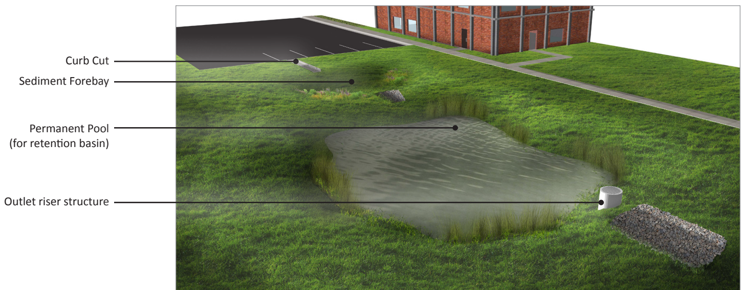
Illustration of a retention basin (permanent pool of water) to capture runoff from adjacent parking lot and in some instances, the adjacent building
